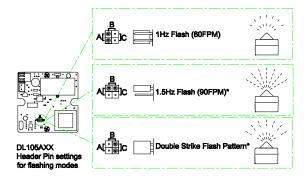
The LED beacon is set as standard to the 2Hz flash mode but it can be set to a steady on mode also. To alter the settings, change the position of the header pin as shown.
