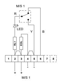
9A - Circuit shown in Unoperated condition (Glass Intact / Standby Condition) Terminals +(2,3) & -(4,5) open Terminals +(2,3) & (6) closed
