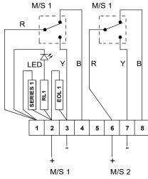
7A - Circuit shown in Unoperated conditi (Glass Intact / Standby Condition) Terminals +(2) & -(3) M/S 1 and +(6) & -(7) M/S Terminals +(2) & (4) M/S 1 and +(6) & (8) M/S 2
