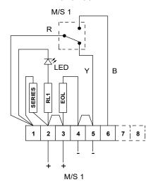
10B - Circuit shown in Operated condition (Glass Broken / Button pushed in) Terminals +(2,3) & -(4,5) closed Terminals +(2,3) & (6) open
