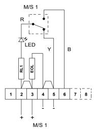
9B - Circuit shown in Operated condition (Glass Broken / Button pushed in) Terminals +(2,3) & -(4,5) closed Terminals +(2,3) & (6) open
