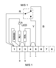
10A - Circuit shown in Unoperated condition (Glass Intact / Standby Condition) Terminals +(2,3) & -(4,5) open Terminals +(2,3) & (6) closed
