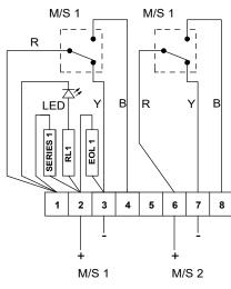
7B - Circuit shown in Operated condition (Glass Broken / Button pushed in) Terminals +(2) & -(3) M/S 1 and +(6) & -(7) M/S 2 Terminals +(2) & (4) M/S 1 and +(6) & (8) M/S 2
