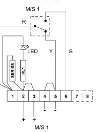
8B - Circuit shown in Operated condition (Glass Broken / Button pushed in) Terminals +(2,3) & -(4,5) closed Terminals +(2,3) & (6) open
