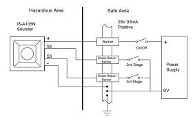
Fig 5 Multi stage alarm using Zener barriers.
