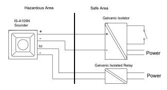
Fig 7 Multi stage alarm using galvanic isolated relays
