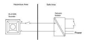
Fig 6 Single stage alarm using galvanic isolator.
