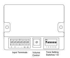
Fig 2 Location of field terminals and controls.
