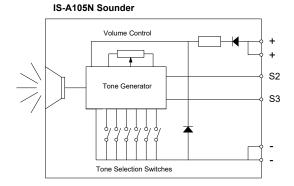
Fig 1 Simplified block diagram
